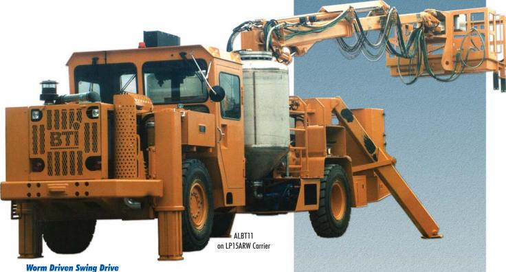
Positive drive for the Turret and Basket Swing c/w spring applied and hydraulic release brakes for smooth operations control and positive hold.
